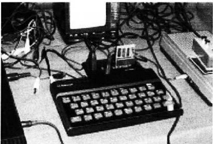
Scotts Selbstbau Speicherinterface Scotts self-built mass storage interface
